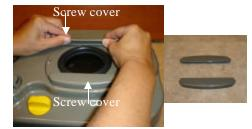
B. Unscrew the 8 screws on the seal cover and, take the seal cover off.
