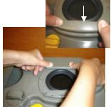
G. Place sliding cover back on its place. Make sure that the two arrows are pointed to each other.
