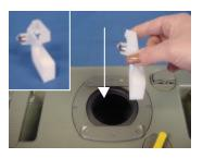
**Note**: If the float retainer is still in the waste tank (float arm has fallen off), the new float arm can not be assembled. Float retainer has to be taken out first. This can be done with a small flat screwdriver. As the waste tank is welded, this can only be done through the hole in the middle.
