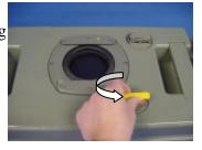
Magnet always has to point to the outside of the waste tank.
