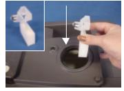
**Note**: If the float retainer is still in the waste tank (float arm has fallen off), the new float arm can not be assembled. Float retainer has to be taken out first. This can be done with a small flat screwdriver. As the waste tank is welded, this can only be done through the hole in the middle.
