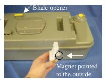
B. For placing the new float arm, take sliding cover off, open the blade and go with your hand in the waste tank.
