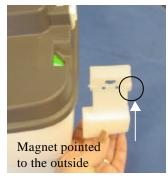
For placing the new float arm, open the B. blade and go with your hand in the waste tank.
